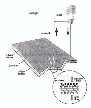
effect on the amount of solar energy received by a photovoltaic array and, in turn, its performance. The efficiency of most commercially available photovoltaic modules in converting sunlight to electricity ranges from 10% to 20%. Researchers around the world are trying to achieve efficiencies up to 50%.
